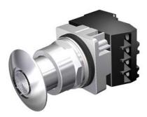
30mm Command/52, Chrome Finish Heavy Duty, Watertight/Oiltight Complete Metal Unit Illuminated Push-Pull Operator Full Voltage, 6V AC LED Lamp Mushroom Head Cap Small 1 3/4" (44.5 mm) Metal, Chrome with Clear Lens 2 Position Maintained, Pull-to-Release with 1 N.O. - 1 N.C. Heavy Duty Contacts, A600/P600 UL Listed, CSA Certified NEMA 1,3,3R,4,4X,12,13 & Automotive Standards
