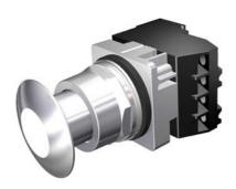
30mm Command/52, Chrome Finish Heavy Duty, Watertight/Oiltight Complete Metal Unit Illuminated Push-Pull Operator Full Voltage, 120V AC/DC LED Lamp Mushroom Head Cap Small 1 3/4" (44.5 mm) Metal, Chrome with White Lens 2 Position Maintained, Pull-to-Release with 1 N.O. - 1 N.C. Heavy Duty Contacts, A600/P600 UL Listed, CSA Certified NEMA 1,3,3R,4,4X,12,13 & Automotive Standards
