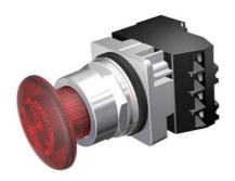
30mm Command/52, Chrome Finish Heavy Duty, Watertight/Oiltight Complete Metal Unit Illuminated Push-Pull Operator Transformer type, 240V AC LED Lamp Mushroom Head Cap Small 1 3/4" (44.5 mm) Plastic, Red 2 Position Maintained, Pull-to-Release with 1 N.O. - 1 N.C. Heavy Duty Contacts, A600/P600 UL Listed, CSA Certified NEMA 1,3,3R,4,4X,12,13 & Automotive Standards
