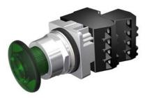
30mm Command/52, Chrome Finish Heavy Duty, Watertight/Oiltight Complete Metal Unit Illuminated Push-Pull Operator Transformer type, 240V AC Incandescent Lamp Mushroom Head Cap Small 1 3/4" (44.5 mm) Plastic, Green 2 Position Maintained, Pull-to-Release with 2 N.O. - 2 N.C. Heavy Duty Contacts, A600/P600 UL Listed, CSA Certified NEMA 1,3,3R,4,4X,12,13 & Automotive Standards
