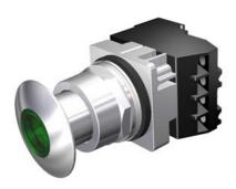
30mm Command/52, Chrome Finish Heavy Duty, Watertight/Oiltight Complete Metal Unit Illuminated Push-Pull Operator Transformer type, 480V AC LED Lamp Mushroom Head Cap Small 1 3/4" (44.5 mm) Metal, Chrome with Green Lens 2 Position Maintained, Pull-to-Release with 1 N.O. - 1 N.C. Heavy Duty Contacts, A600/P600 UL Listed, CSA Certified NEMA 1,3,3R,4,4X,12,13 & Automotive Standards
