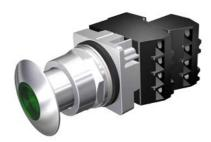
30mm Command/52, Chrome Finish Heavy Duty, Watertight/Oiltight Complete Metal Unit Illuminated Push-Pull Operator Transformer type, 480V AC Incandescent Lamp Mushroom Head Cap Small 1 3/4" (44.5 mm) Metal, Chrome with Green Lens 2 Position Maintained, Pull-to-Release with 2 N.O. - 2 N.C. Heavy Duty Contacts, A600/P600 UL Listed, CSA Certified NEMA 1,3,3R,4,4X,12,13 & Automotive Standards
