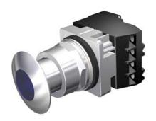
30mm Command/52, Chrome Finish Heavy Duty, Watertight/Oiltight Complete Metal Unit Illuminated Push-Pull Operator Transformer type, 480V AC LED Lamp Mushroom Head Cap Small 1 3/4" (44.5 mm) Metal, Chrome with Blue Lens 2 Position Maintained, Pull-to-Release with 1 N.O. - 1 N.C. Heavy Duty Contacts, A600/P600 UL Listed, CSA Certified NEMA 1,3,3R,4,4X,12,13 & Automotive Standards
