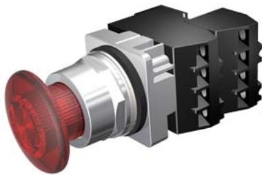
30mm Command/52, Chrome Finish Heavy Duty, Watertight/Oiltight Complete Metal Unit Illuminated Push-Pull Operator Transformer type, 480V AC Incandescent Lamp Mushroom Head Cap Small 1 3/4" (44.5 mm) Plastic, Red 2 Position Maintained, Pull-to-Release with 2 N.O. - 2 N.C. Heavy Duty Contacts, A600/P600 UL Listed, CSA Certified NEMA 1,3,3R,4,4X,12,13 & Automotive Standards
