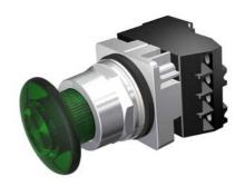
30mm Command/52, Chrome Finish Heavy Duty,Watertight/Oiltight Complete Metal Unit Illuminated Push-Pull Operator Transformer type, 480V AC LED Lamp Mushroom Head Cap Small 1 3/4" (44.5 mm) Plastic, Green 2 Position Maintained, Pull-to-Release with 1 N.O. - 1 N.C. Heavy Duty Contacts, A600/P600 UL Listed, CSA Certified NEMA 1,3,3R,4,4X,12,13 & Automotive Standards
