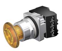
30mm Command/52, Chrome Finish Heavy Duty,Watertight/Oiltight Complete Metal Unit Illuminated Push-Pull Operator Transformer type, 480V AC LED Lamp Mushroom Head Cap Small 1 3/4" (44.5 mm) Plastic, Amber 2 Position Maintained, Pull-to-Release with 1 N.O. - 1 N.C. Heavy Duty Contacts, A600/P600 UL Listed, CSA Certified NEMA 1,3,3R,4,4X,12,13 & Automotive Standards
