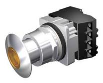
30mm Command/52, Chrome Finish Heavy Duty,Watertight/Oiltight Complete Metal Unit Illuminated Push-Pull Operator Transformer type, 600V AC LED Lamp Mushroom Head Cap Small 1 3/4" (44.5 mm) Metal, Chrome with Amber Lens 2 Position Maintained, Pull-to-Release with 1 N.O. - 1 N.C. Heavy Duty Contacts, A600/P600 UL Listed, CSA Certified NEMA 1,3,3R,4,4X,12,13 & Automotive Standards
