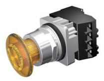
30mm Command/52, Chrome Finish Heavy Duty, Watertight/Oiltight Complete Metal Unit Illuminated Push-Pull Operator Transformer type, 600V AC LED Lamp Mushroom Head Cap Small 1 3/4" (44.5 mm) Plastic, Amber 2 Position Maintained, Pull-to-Release with 1 N.O. - 1 N.C. Heavy Duty Contacts, A600/P600 UL Listed, CSA Certified NEMA 1,3,3R,4,4X,12,13 & Automotive Standards
