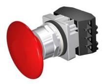
30mm Command/52, Chrome Finish Heavy Duty, Watertight/Oiltight Complete Metal Unit Push-Pull Operator Non-Illuminated Mushroom Head Cap Large 2 1/2" (63.5 mm) Plastic, Red 2 Position Maintained, Pull-to-Release with 2 N.O. - 2 N.C. Heavy Duty Contacts, A600/P600 UL Listed, CSA Certified NEMA 1,3,3R,4,4X,12,13 & Automotive Standards
