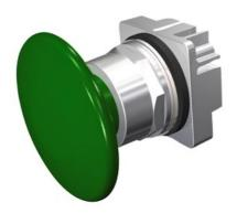
30mm Command/52, Chrome Finish Heavy Duty, Watertight/Oiltight Metal Operator, Round Push-Pull Operator Non-Illuminated Mushroom Head Cap Large 2 1/2" (63.5 mm) Plastic, Green 2 Position Maintained, Pull-to-Release UL Listed, CSA Certified NEMA 1,3,3R,4,4X,12,13 & Automotive Standards
