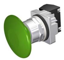
30mm Command/52, Chrome Finish Heavy Duty,Watertight/Oiltight Complete Metal Unit Push-Pull Operator Non-Illuminated Mushroom Head Cap Large 2 1/2" (63.5 mm) Plastic, Green 2 Position Maintained, Pull-to-Release with 1 N.O. - 1 N.C. Heavy Duty Contacts, A600/P600 UL Listed, CSA Certified NEMA 1,3,3R,4,4X,12,13 & Automotive Standards
