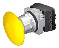
30mm Command/52, Chrome Finish Heavy Duty, Watertight/Oiltight Complete Metal Unit Push-Pull Operator Non-Illuminated Mushroom Head Cap Large 2 1/2" (63.5 mm) Plastic, Yellow 2 Position Maintained, Pull-to-Release with 2 N.O. - 2 N.C. Heavy Duty Contacts, A600/P600 UL Listed, CSA Certified NEMA 1,3,3R,4,4X,12,13 & Automotive Standards
