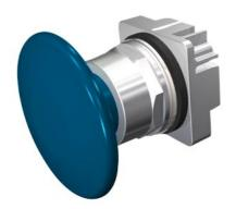
30mm Command/52, Chrome Finish Heavy Duty, Watertight/Oiltight Metal Operator, Round Push-Pull Operator Non-Illuminated Mushroom Head Cap Large 2 1/2" (63.5 mm) Plastic, Blue 2 Position Maintained, Pull-to-Release UL Listed, CSA Certified NEMA 1,3,3R,4,4X,12,13 & Automotive Standards
