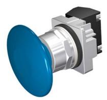
30mm Command/52, Chrome Finish Heavy Duty,Watertight/Oiltight Complete Metal Unit Push-Pull Operator Non-Illuminated Mushroom Head Cap Large 2 1/2" (63.5 mm) Plastic, Blue 2 Position Maintained, Pull-to-Release with 1 N.O. - 1 N.C. Heavy Duty Contacts, A600/P600 UL Listed, CSA Certified NEMA 1,3,3R,4,4X,12,13 & Automotive Standards
