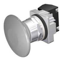
30mm Command/52, Chrome Finish Heavy Duty,Watertight/Oiltight Complete Metal Unit Push-Pull Operator Non-Illuminated Mushroom Head Cap Large 2 1/2" (63.5 mm) Plastic, Gray 2 Position Maintained, Pull-to-Release with 1 N.O. - 1 N.C. Heavy Duty Contacts, A600/P600 UL Listed, CSA Certified NEMA 1,3,3R,4,4X,12,13 & Automotive Standards
