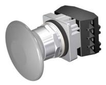
30mm Command/52, Chrome Finish Heavy Duty,Watertight/Oiltight Complete Metal Unit Push-Pull Operator Non-Illuminated Mushroom Head Cap Large 2 1/2" (63.5 mm) Plastic, Gray 2 Position Maintained, Pull-to-Release with 2 N.O. - 2 N.C. Heavy Duty Contacts, A600/P600 UL Listed, CSA Certified NEMA 1,3,3R,4,4X,12,13 & Automotive Standards
