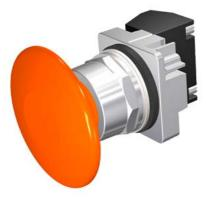
30mm Command/52, Chrome Finish Heavy Duty, Watertight/Oiltight Complete Metal Unit Push-Pull Operator Non-Illuminated Mushroom Head Cap Large 2 1/2" (63.5 mm) Plastic, Orange 2 Position Maintained, Pull-to-Release with 1 N.O. - 1 N.C. Heavy Duty Contacts, A600/P600 UL Listed, CSA Certified NEMA 1,3,3R,4,4X,12,13 & Automotive Standards
