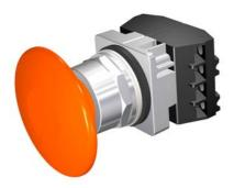
30mm Command/52, Chrome Finish Heavy Duty, Watertight/Oiltight Complete Metal Unit Push-Pull Operator Non-Illuminated Mushroom Head Cap Large 2 1/2" (63.5 mm) Plastic, Orange 2 Position Maintained, Pull-to-Release with 2 N.O. - 2 N.C. Heavy Duty Contacts, A600/P600 UL Listed, CSA Certified NEMA 1,3,3R,4,4X,12,13 & Automotive Standards
