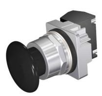
30mm Command/52, Chrome Finish Heavy Duty,Watertight/Oiltight Complete Metal Unit Push-Pull Operator Non-Illuminated Mushroom Head Cap Small 1 3/4" (44.5 mm) Plastic, Black 2 Position Maintained, Pull-to-Release with 1 N.O. - 1 N.C. Heavy Duty Contacts, A600/P600 UL Listed, CSA Certified NEMA 1,3,3R,4,4X,12,13 & Automotive Standards
