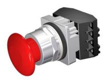
30mm Command/52, Chrome Finish Heavy Duty,Watertight/Oiltight Complete Metal Unit Push-Pull Operator Non-Illuminated Mushroom Head Cap Small 1 3/4" (44.5 mm) Plastic, Red 2 Position Maintained, Pull-to-Release with 2 N.O. - 2 N.C. Heavy Duty Contacts, A600/P600 UL Listed, CSA Certified NEMA 1,3,3R,4,4X,12,13 & Automotive Standards
