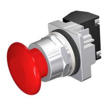
30mm Command/52, Chrome Finish Heavy Duty,Watertight/Oiltight Complete Metal Unit Push-Pull Operator Non-Illuminated Mushroom Head Cap Small 1 3/4" (44.5 mm) Plastic, Red 2 Position Maintained, Pull-to-Release with 1 N.C. Heavy Duty Contacts, A600/P600 UL Listed, CSA Certified NEMA 1,3,3R,4,4X,12,13 & Automotive Standards
