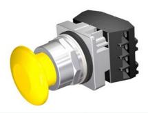
30mm Command/52, Chrome Finish Heavy Duty, Watertight/Oiltight Complete Metal Unit Push-Pull Operator Non-Illuminated Mushroom Head Cap Small 1 3/4" (44.5 mm) Plastic, Yellow 2 Position Maintained, Pull-to-Release with 2 N.O. - 2 N.C. Heavy Duty Contacts, A600/P600 UL Listed, CSA Certified NEMA 1,3,3R,4,4X,12,13 & Automotive Standards
