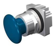
30mm Command/52, Chrome Finish Heavy Duty, Watertight/Oiltight Metal Operator, Round Push-Pull Operator Non-Illuminated Mushroom Head Cap Small 1 3/4" (44.5 mm) Plastic, Blue 2 Position Maintained, Pull-to-Release UL Listed, CSA Certified NEMA 1,3,3R,4,4X,12,13 & Automotive Standards
