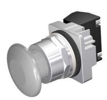
30mm Command/52, Chrome Finish Heavy Duty,Watertight/Oiltight Complete Metal Unit Push-Pull Operator Non-Illuminated Mushroom Head Cap Small 1 3/4" (44.5 mm) Plastic, Gray 2 Position Maintained, Pull-to-Release with 1 N.O. - 1 N.C. Heavy Duty Contacts, A600/P600 UL Listed, CSA Certified NEMA 1,3,3R,4,4X,12,13 & Automotive Standards
