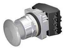
30mm Command/52, Chrome Finish Heavy Duty,Watertight/Oiltight Complete Metal Unit Push-Pull Operator Non-Illuminated Mushroom Head Cap Small 1 3/4" (44.5 mm) Plastic, Gray 2 Position Maintained, Pull-to-Release with 2 N.O. - 2 N.C. Heavy Duty Contacts, A600/P600 UL Listed, CSA Certified NEMA 1,3,3R,4,4X,12,13 & Automotive Standards
