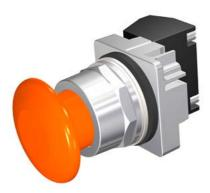
30mm Command/52, Chrome Finish Heavy Duty, Watertight/Oiltight Complete Metal Unit Push-Pull Operator Non-Illuminated Mushroom Head Cap Small 1 3/4" (44.5 mm) Plastic, Orange 2 Position Maintained, Pull-to-Release with 1 N.O. - 1 N.C. Heavy Duty Contacts, A600/P600 UL Listed, CSA Certified NEMA 1,3,3R,4,4X,12,13 & Automotive Standards
