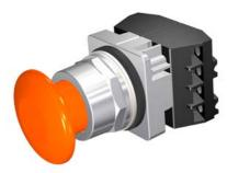
30mm Command/52, Chrome Finish Heavy Duty, Watertight/Oiltight Complete Metal Unit Push-Pull Operator Non-Illuminated Mushroom Head Cap Small 1 3/4" (44.5 mm) Plastic, Orange 2 Position Maintained, Pull-to-Release with 2 N.O. - 2 N.C. Heavy Duty Contacts, A600/P600 UL Listed, CSA Certified NEMA 1,3,3R,4,4X,12,13 & Automotive Standards
