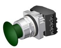
30mm Command/52, Chrome Finish Heavy Duty,Watertight/Oiltight Complete Metal Unit Push-Pull Operator Non-Illuminated Mushroom Head Cap Small 1.73" (44 mm) Metal, Anodized Green 3 Position Momentary 1 N.C.+1 N.C. Extra Late Break Heavy Duty Contacts, A600/P600 UL Listed, CSA Certified NEMA 1,3,3R,4,4X,12,13 & Automotive Standards
