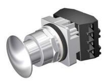
30mm Command/52, Chrome Finish Heavy Duty, Watertight/Oiltight Complete Metal Unit Push-Pull Operator Non-Illuminated Mushroom Head Cap Small 1.73" (44 mm) Metal, Chrome 3 Position Momentary 1 N.C.+1 N.C. Extra Late Break Heavy Duty Contacts, A600/P600 UL Listed, CSA Certified NEMA 1,3,3R,4,4X,12,13 & Automotive Standards
