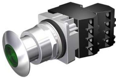
30mm Command/52, Chrome Finish Heavy Duty, Watertight/Oiltight Complete Metal Unit Illuminated Push-Pull Operator Full Voltage, 12V AC/DC Incandescent Lamp Mushroom Head Cap Small 1 3/4" (44.5 mm) Metal, Chrome with Green Lens 3 Position Momentary 1 N.C.+1 N.C. Extra Late Break Heavy Duty Contacts, A600/P600 UL Listed, CSA Certified NEMA 1,3,3R,4,4X,12,13 & Automotive Standards
