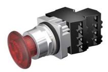
30mm Command/52, Chrome Finish Heavy Duty, Watertight/Oiltight Complete Metal Unit Illuminated Push-Pull Operator Transformer type, 120V AC Incandescent Lamp Mushroom Head Cap Small 1 3/4" (44.5 mm) Plastic, Red 3 Position Momentary 1 N.C.+1 N.C. Extra Late Break Heavy Duty Contacts, A600/P600 UL Listed, CSA Certified NEMA 1,3,3R,4,4X,12,13 & Automotive Standards
