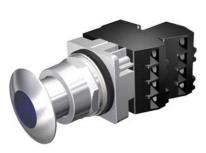
30mm Command/52, Chrome Finish Heavy Duty,Watertight/Oiltight Complete Metal Unit Illuminated Push-Pull Operator Transformer type, 480V AC LED Lamp Mushroom Head Cap Small 1 3/4" (44.5 mm) Metal, Chrome with Blue Lens 3 Position Momentary 1 N.C.+1 N.C. Extra Late Break Heavy Duty Contacts, A600/P600 UL Listed, CSA Certified NEMA 1,3,3R,4,4X,12,13 & Automotive Standards
