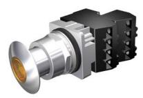
30mm Command/52, Chrome Finish Heavy Duty, Watertight/Oiltight Complete Metal Unit Illuminated Push-Pull Operator Transformer type, 480V AC Incandescent Lamp Mushroom Head Cap Small 1 3/4" (44.5 mm) Metal, Chrome with Amber Lens 3 Position Momentary 1 N.C.+1 N.C. Extra Late Break Heavy Duty Contacts, A600/P600 UL Listed, CSA Certified NEMA 1,3,3R,4,4X,12,13 & Automotive Standards
