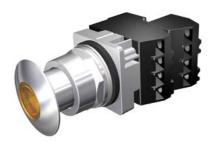
30mm Command/52, Chrome Finish Heavy Duty,Watertight/Oiltight Complete Metal Unit Illuminated Push-Pull Operator Transformer type, 480V AC LED Lamp Mushroom Head Cap Small 1 3/4" (44.5 mm) Metal, Chrome with Amber Lens 3 Position Momentary 1 N.C.+1 N.C. Extra Late Break Heavy Duty Contacts, A600/P600 UL Listed, CSA Certified NEMA 1,3,3R,4,4X,12,13 & Automotive Standards
