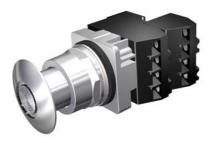
30mm Command/52, Chrome Finish Heavy Duty, Watertight/Oiltight Complete Metal Unit Illuminated Push-Pull Operator Transformer type, 480V AC LED Lamp Mushroom Head Cap Small 1 3/4" (44.5 mm) Metal, Chrome with Clear Lens 3 Position Momentary 1 N.C.+1 N.C. Extra Late Break Heavy Duty Contacts, A600/P600 UL Listed, CSA Certified NEMA 1,3,3R,4,4X,12,13 & Automotive Standards
