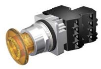
30mm Command/52, Chrome Finish Heavy Duty, Watertight/Oiltight Complete Metal Unit Illuminated Push-Pull Operator Transformer type, 480V AC Incandescent Lamp Mushroom Head Cap Small 1 3/4" (44.5 mm) Plastic, Amber 3 Position Momentary 1 N.C.+1 N.C. Extra Late Break Heavy Duty Contacts, A600/P600 UL Listed, CSA Certified NEMA 1,3,3R,4,4X,12,13 & Automotive Standards
