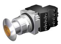
30mm Command/52, Chrome Finish Heavy Duty,Watertight/Oiltight Complete Metal Unit Illuminated Push-Pull Operator Transformer type, 600V AC LED Lamp Mushroom Head Cap Small 1 3/4" (44.5 mm) Metal, Chrome with Amber Lens 3 Position Momentary 1 N.C.+1 N.C. Extra Late Break Heavy Duty Contacts, A600/P600 UL Listed, CSA Certified NEMA 1,3,3R,4,4X,12,13 & Automotive Standards
