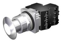
30mm Command/52, Chrome Finish Heavy Duty, Watertight/Oiltight Complete Metal Unit Illuminated Push-Pull Operator Transformer type, 600V AC Incandescent Lamp Mushroom Head Cap Small 1 3/4" (44.5 mm) Metal, Chrome with White Lens 3 Position Momentary 1 N.C.+1 N.C. Extra Late Break Heavy Duty Contacts, A600/P600 UL Listed, CSA Certified NEMA 1,3,3R,4,4X,12,13 & Automotive Standards
