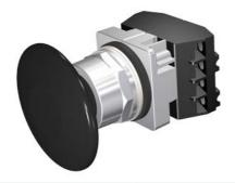
30mm Command/52, Chrome Finish Heavy Duty, Watertight/Oiltight Complete Metal Unit Push-Pull Operator Non-Illuminated Mushroom Head Cap Large 2 1/2" (63.5 mm) Plastic, Black 3 Position Momentary 1 N.C.+1 N.C. Extra Late Break Heavy Duty Contacts, A600/P600 UL Listed, CSA Certified NEMA 1,3,3R,4,4X,12,13 & Automotive Standards
