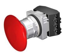
30mm Command/52, Chrome Finish Heavy Duty,Watertight/Oiltight Complete Metal Unit Push-Pull Operator Non-Illuminated Mushroom Head Cap Large 2 1/2" (63.5 mm) Plastic, Red 3 Position Momentary 1 N.C.+1 N.C. Extra Late Break Heavy Duty Contacts, A600/P600 UL Listed, CSA Certified NEMA 1,3,3R,4,4X,12,13 & Automotive Standards
