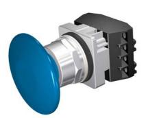
30mm Command/52, Chrome Finish Heavy Duty,Watertight/Oiltight Complete Metal Unit Push-Pull Operator Non-Illuminated Mushroom Head Cap Large 2 1/2" (63.5 mm) Plastic, Blue 3 Position Momentary 1 N.C.+1 N.C. Extra Late Break Heavy Duty Contacts, A600/P600 UL Listed, CSA Certified NEMA 1,3,3R,4,4X,12,13 & Automotive Standards
