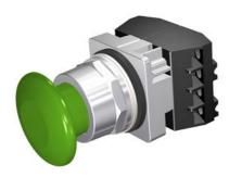
30mm Command/52, Chrome Finish Heavy Duty,Watertight/Oiltight Complete Metal Unit Push-Pull Operator Non-Illuminated Mushroom Head Cap Small 1 3/4" (44.5 mm) Plastic, Green 3 Position Momentary 1 N.C.+1 N.C. Extra Late Break Heavy Duty Contacts, A600/P600 UL Listed, CSA Certified NEMA 1,3,3R,4,4X,12,13 & Automotive Standards
