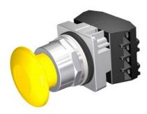
30mm Command/52, Chrome Finish Heavy Duty,Watertight/Oiltight Complete Metal Unit Push-Pull Operator Non-Illuminated Mushroom Head Cap Small 1 3/4" (44.5 mm) Plastic, Yellow 3 Position Momentary 1 N.C.+1 N.C. Extra Late Break Heavy Duty Contacts, A600/P600 UL Listed, CSA Certified NEMA 1,3,3R,4,4X,12,13 & Automotive Standards
