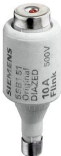
DIAZED FUSE LINK 500V QUICK-RESPONSE SIZE DII, THREAD E27, 10A
