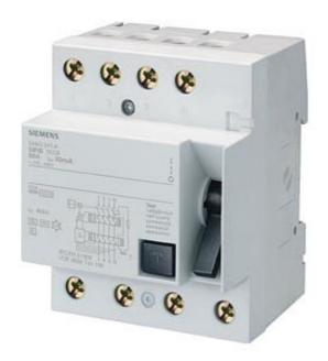
RES.CURR. OP.CIRC. BR. SIQUENCE TYPE B SENS. TO. UNIV. CURRENT 40A 3+N-POL IFN 30MA 400V 4MW SHORT-TIME DELAYED
