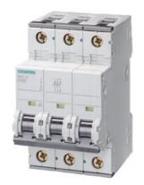
Miniature circuit breaker 400 V D=70 mm 25 kA according to EN 60947-2, 3P, D6
